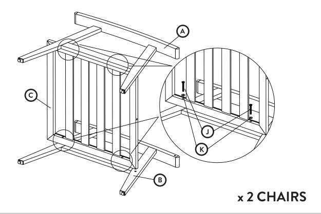
STEP 2 Using the M6x20mm bolts (I), M6x55mm bolts (J) and washers (K), attach the chair back (D) to the chair bottom (C), and the left and right arms (A,B).
